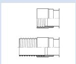
Flanged pipe according to the popular pipe systems in the ventilation field (for example Jacob-Standard), food-grade
