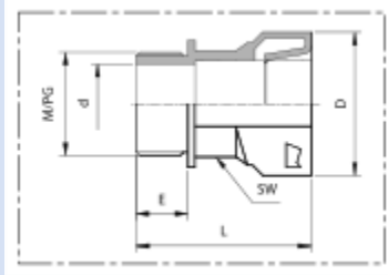
Plastic conduit connector; rigid connecting thread
